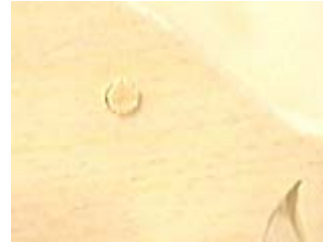
Insert them in the hole with the grain running in the same direction
