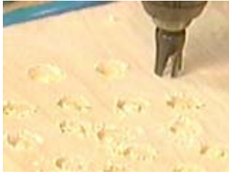
Use a plug cutter to make plugs from your project wood
