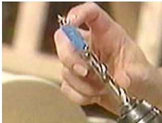
Using a brad point bit makes a clean hole for a plug
